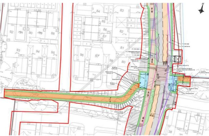
These show that only a small diversion needs to take place. This is to provide a safe and level crossing of the new spine road through the NW Cullompton Urban Extension and we have worked to ensure that the minimum diversion possible is being proposed, and to ensure that the new route is planted with trees and hedges. The diversion is required for the development to take place. Alternatives have been considered and they do not work in terms of road and bridleway safety.
